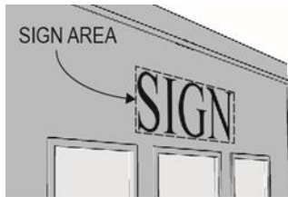
Figure 5:22-4 Wall Sign without panel
